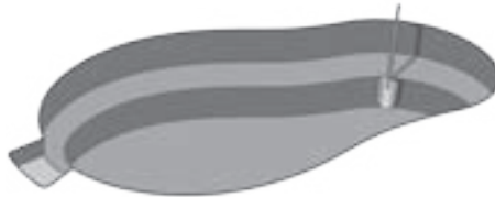
Fig. 4 Dig second shelf one shovel depth and start excavation of skimmer hole.
