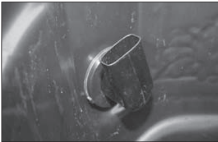
Fig. 33 Dial-in the adjustable overflow arm.
