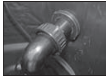
Fig. 23 One adaptor threads directly into the pump, the other threads directly into the bulkhead on the back of the skimmer.
