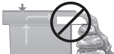
Fig. 13 If a thick rock along with a larger flow pump is used, the water flow may be so great that it will flow over the sides of the MicroFalls® filter.
